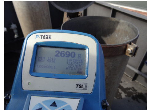
Particulate counter shows very low UFP concentration directly next to the smoke stack. Foto:NABU/Diesener
